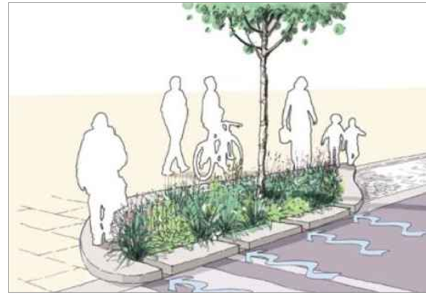
FIGURES 2 & 3: NATURE-BASED SOLUTIONS (NB SUDs) RAIN GARDENS DRAINAGE SOLUTIONS FOR LANDSCAPING
